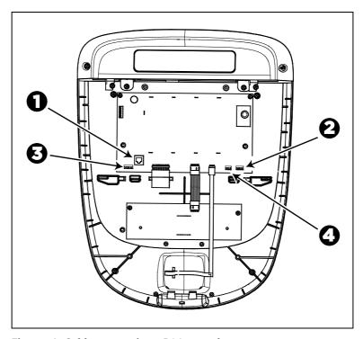
Figure 18: Cable connections, P20 console
